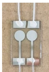
Figure 1 : Schematic and photograph of the glass substrate used in the interconnection tests
