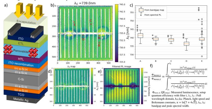
Figure 1– a) Perovskite/silicon tandem stack, b) perovskite top-cell bandgap map, c) bandgap map extractions compared to spectrometer measurements, d) perovskite top-cell bandgap width and e) regular PL image, f) semi-physical model
